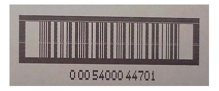
Problem: Missing channels and channel fractures in print channels.
