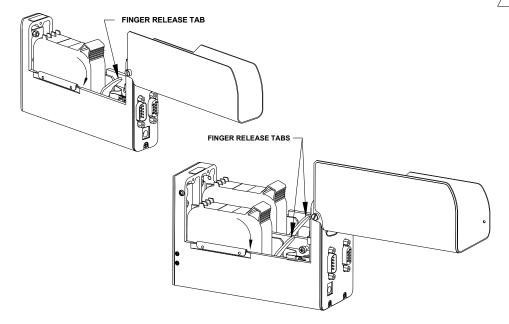
When inserting cartridge, aim nose at an angle towards black pogo pin component. Slide pen cartridge up to Pen Stop.
