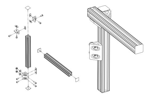
**Step 2: Assemble Bracketry to Conveyor**
