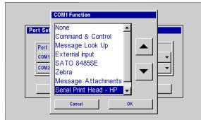
If using a PC, pressing OK after selecting Serial Print Head-HP opens the Serial Port Setup dialog box. Select the desired COM port (only those ports available are listed) and press OK. Press OK again to exit the Port Settings Screen.
