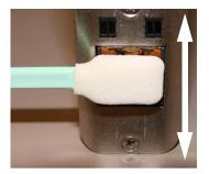
Wipe pen cartridge face up and down several times. Immediately press and hold the purge button for 5-10 seconds.
