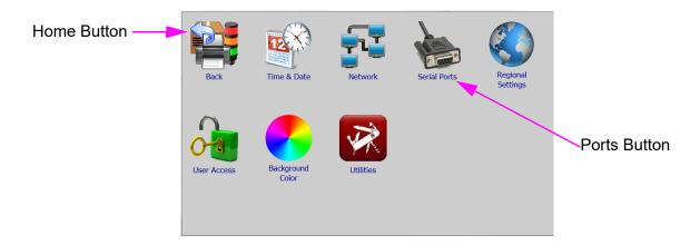
On the Ports Setting Screen press the **COM1** Function Button, select **Serial Print Head-HP**, and press OK. Press OK again to exit the Port Settings Screen.
