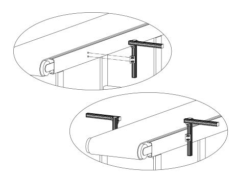
**Step 3: Assemble Print Head and Power Supply to Bracketry**
