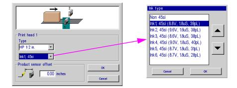
Print head setup complete. Next, select the **Encoder** tab and choose the desired encoder type.
