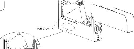
3. Rotate Pen Cartridge down until it snaps in place.
