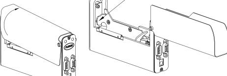
2. Insert Pen Cartridge at an angle up to Pen Stop
