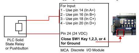
Connection to PLC triggering MCA input, PLC Sourcing Power
