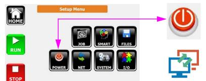
Pressing the power button will do a soft power off. When the system shuts down it can be awakened by pressing anywhere on the display.
