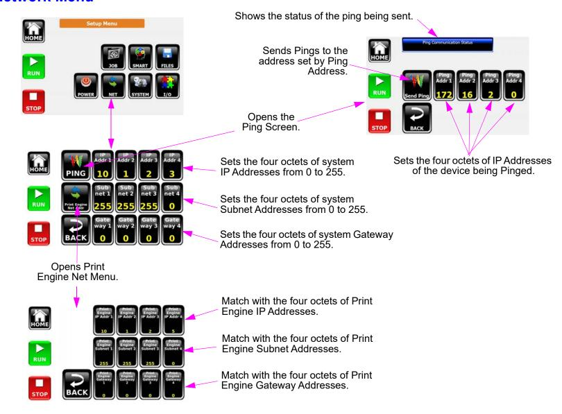
**NOTE:** Print Engine Net Address menu does not set the address for the print engine. The Print Engine Net Address should be set in the print engine.
