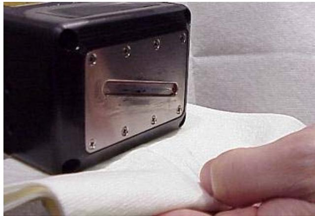
3. Wipe the excess ink from the front plate with a lint-free wipe. Run another test print using the print/purge feature while swiping a lint-free cloth vertically in front of the head. Inspect for all 32 channels printing. Repeat the priming process and test printing until all 32 channels print.
