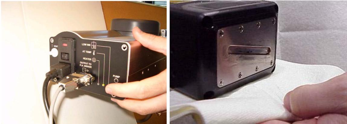
2. Wipe the excess ink from the front plate with a lint-free wipe. Run another test print. Inspect for all 32 channels printing. Repeat the priming process and test printing until all 32 channels print.
