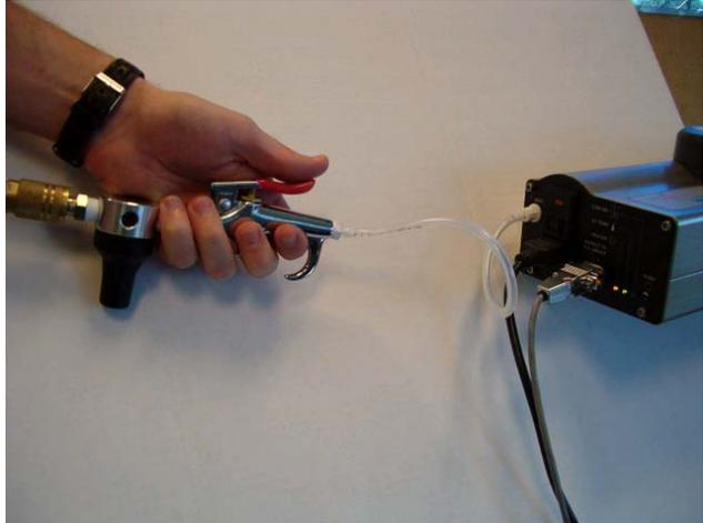
2. A lint-free wipe must be placed in front of the orifice plate to collect the ink expelled from the front plate.
