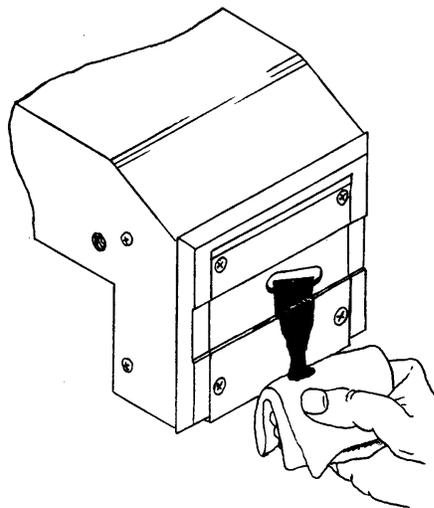
2. Insert the priming bulb into the reservoir (do not plug the hole in the bulb) and squeeze 2 or 3 times. Wax should flow out of the nozzles. Wipe faceplate gently while avoiding wiping the Array Plate.
