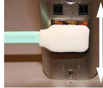
Wipe pen cartridge face up and down several times. Immediately press and hold the purge button for 5-10 seconds.
