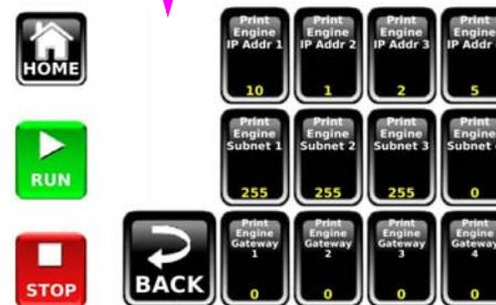
Match with the four octets of Print Engine IP Addresses.
