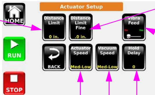
The furthest extension of the tamp with 6mm (1/4") increments.
