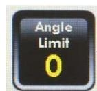
The furthest swing angle for E-FASA application instead of Distance Limit.
