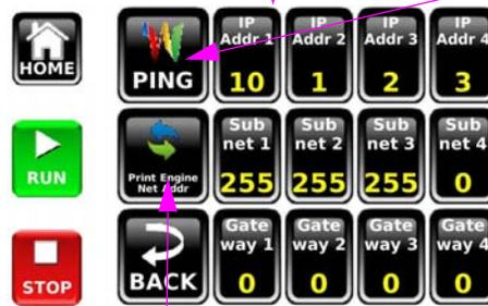
Sets the four octets of system IP Addresses from 0 to 255.
